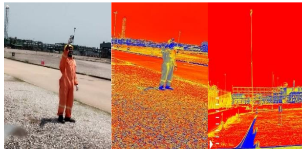
Figure 2: Facility B methane monitoring and dispersion under infrared camera
